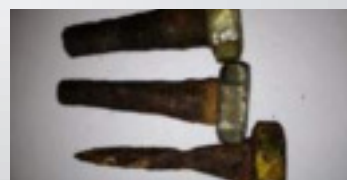
These rusted bolts were all that was securing a 200 gallon power sprayer. Inspect for this – use quality stainless steel bolts & nylock nuts to prevent hardware from vibrating off.
