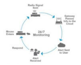
Kness has introduced its own version of a remote monitoring system called KritterSense. It is a small sensor unit, about the size
